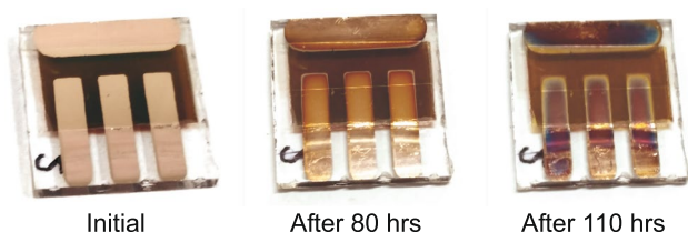
Fig. 9 Photographs of a Cu electrode based PSC taken after different time intervals. The solar cell was not encapsulated and stored in dark. The oxidation of top Cu electrode with time could be seen clearly by the change in its surface color
