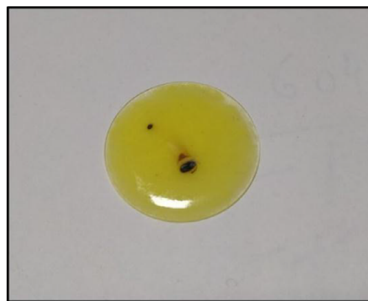
Figure 4. Phosphor-epoxy layer without integrating sapphire. The optical image clearly exhibits burning of the sample after exposure with blue laser (0.8 W) beam.
