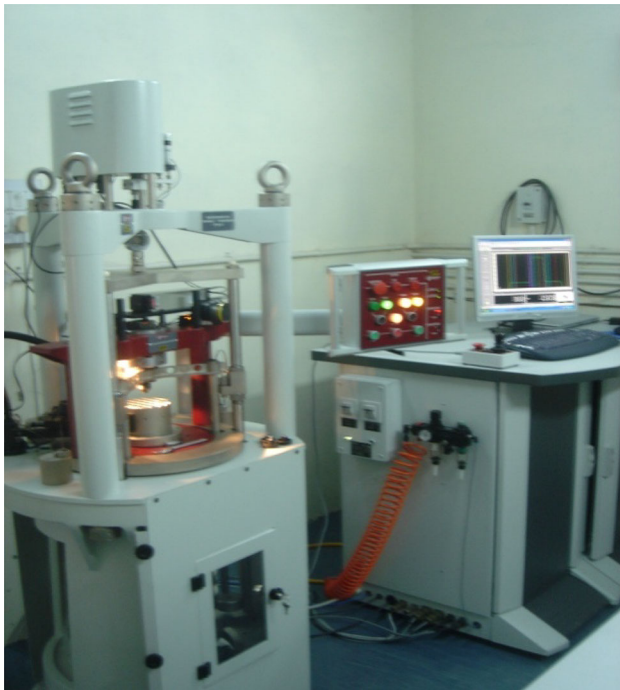
Fig. 2 Primary Vickers hardness machine at CSIR-NPL, New Delhi
