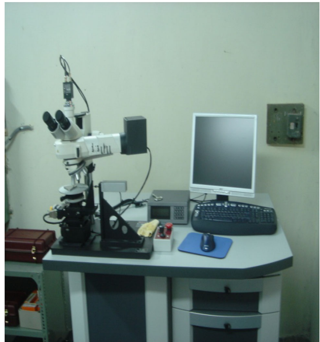
Fig. 3 Indentation diagonal measuring system associated with the primary Vickers hardness machine at CSIR-NPL
