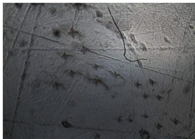
Fig. 7. Vickers indentation mark on doped SA crystal at different loads.
